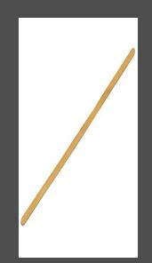
• A rod is used to manually stir solutions. It can also be used to transfer a single drop of a solution. • Can be glass, plastic or wood.
