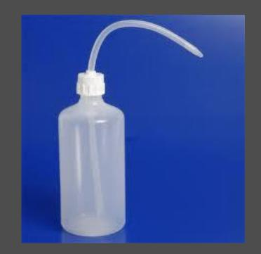
A wash bottle has a spout that delivers a wash solution to a specific area. Distilled water should be used in a wash bottle. IT IS NOT FOR WASHING EQUIPMENT OR CLEANING!!!
