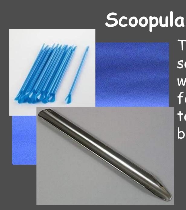
Transfer solids: to a weigh paper for weighing, to a weighing boat.
