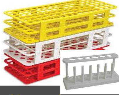
Test tube racks are for holding and organizing test tubes on the laboratory counter. Plastic racks may melt in contact with very hot test tubes. Can be plastic, wood or metal.
