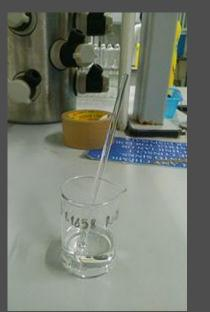
manually stir solutions. It can also be used to transfer a single drop of a solution. • Can be glass, plastic or wood.
