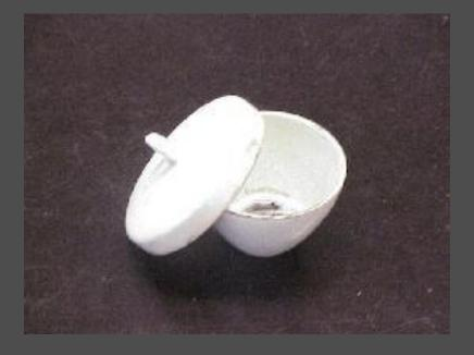
Crucibles are used for heating certain solids, particularly metals, to very high temperatures.
