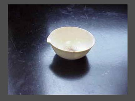
The evaporating dish is used for the heating of stable solid compounds and elements.
