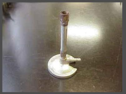
Bunsen burners are used for the heating of nonvolatile liquids and solids.
