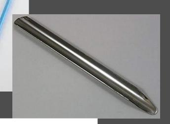
Transfer solids: to a weigh paper for weighing, to a weighing boat.
