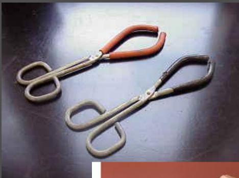
Beaker tongs are used to move beakers containing hot liquids.
