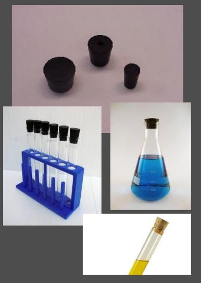
Rubber stoppers are used to close containers & test tubes to avoid spillage or contamination. Containers should never be heated when there is a stopper in place.
