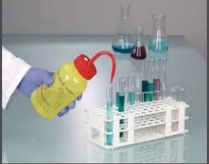
A wash bottle has a spout that delivers a wash solution to a specific area. Distilled water should be used in a wash bottle. • IT IS NOT FOR WASHING EQUIPMENT OR CLEANING!!!
